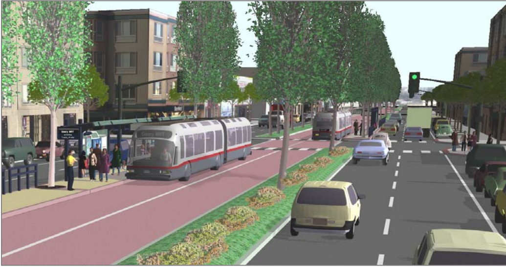
Figure 12. Conceptual Simulation of Center-Running BRT with Side Platforms / Dual Medians
