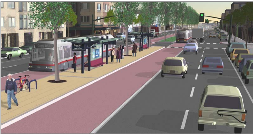
Figure 13. Conceptual Simulation of Center-Running BRT with Center Platforms
