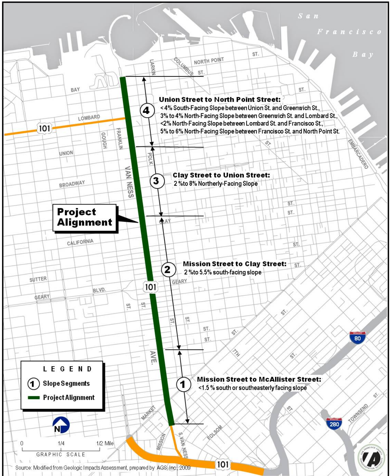
Figure 4.7-1: Project Alignment Slope Map
