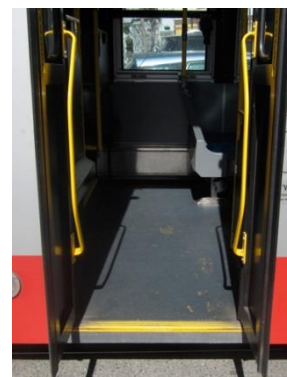
Buses with low floors speed up boarding time by reducing the number of steps required to board the bus.
