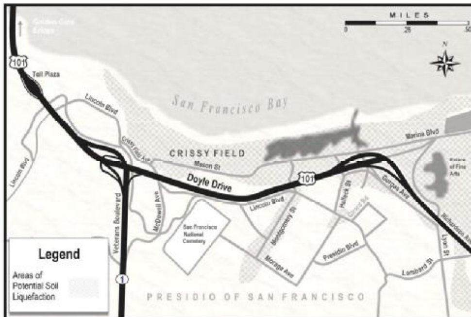
Exhibit 3-52 Potential Areas of Soil Liquefaction
