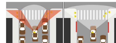
Daylighting at intersection
