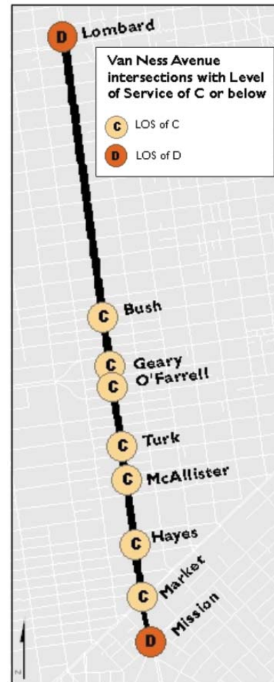
Figure 2-18: Van Ness Intersection Operation
