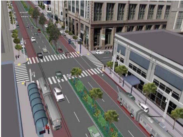
Figure 3-18: Alternative 2, Curb Lane BRT, at Geary/O'Farrell
