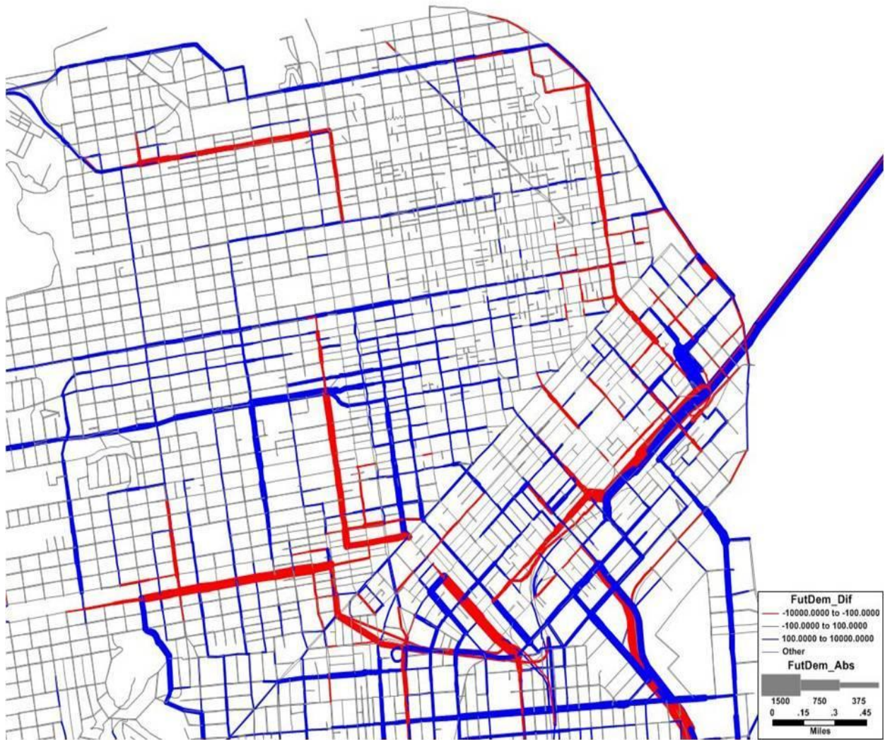
Figure 21. Flow Difference Map from 5:00 to 6:00 pm in CBD for 2040 Demand Test (Red links- decrease of at least 100 vehicles, Blue links - increase of at least 100 vehicles)
