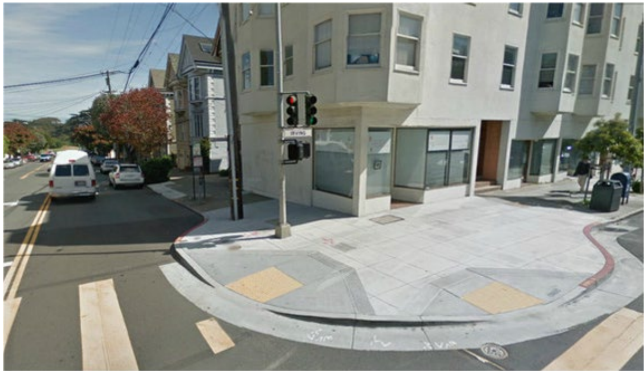
Typical After – Bulb-out
