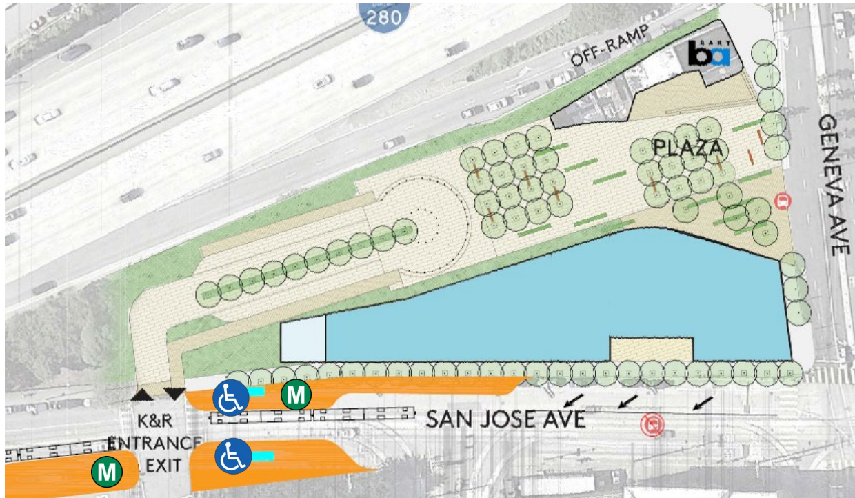
Figure 8 – Recommended Alternative, incorporating future BART Plaza, drop off loop and Upper Yard development
