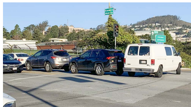
Westbound queued vehicles block northbound off-ramp left turns.
