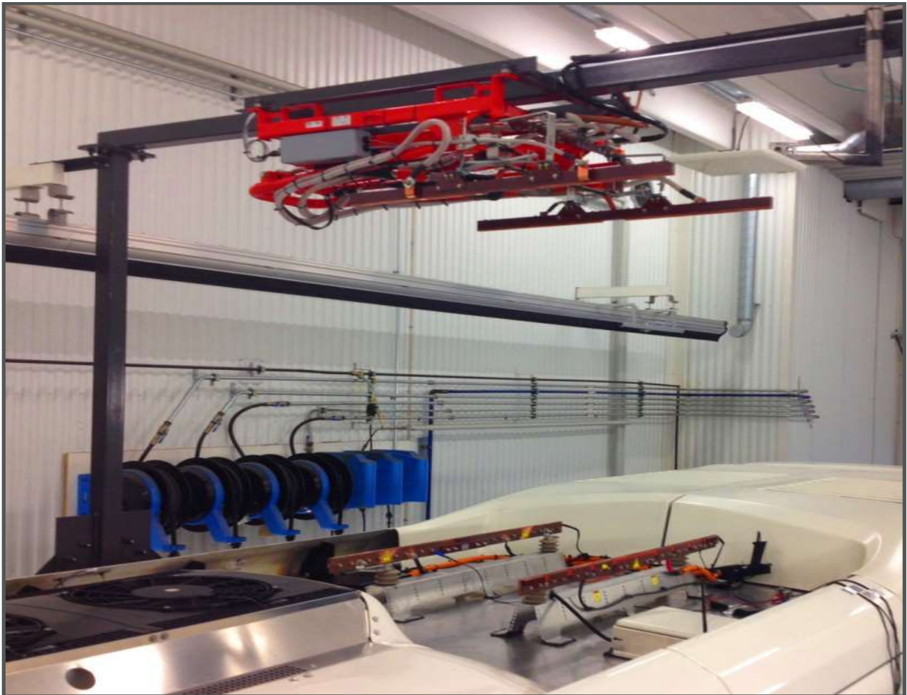
Figure 3-1. Inverted Pantograph and Charge Rails
