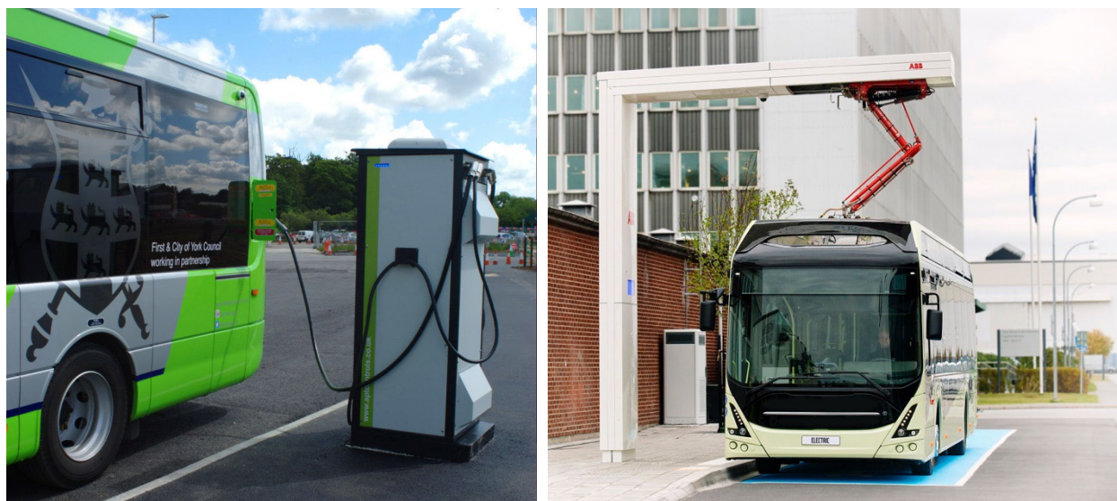
Figure 2-1. Plug-In and Pantograph Charging
