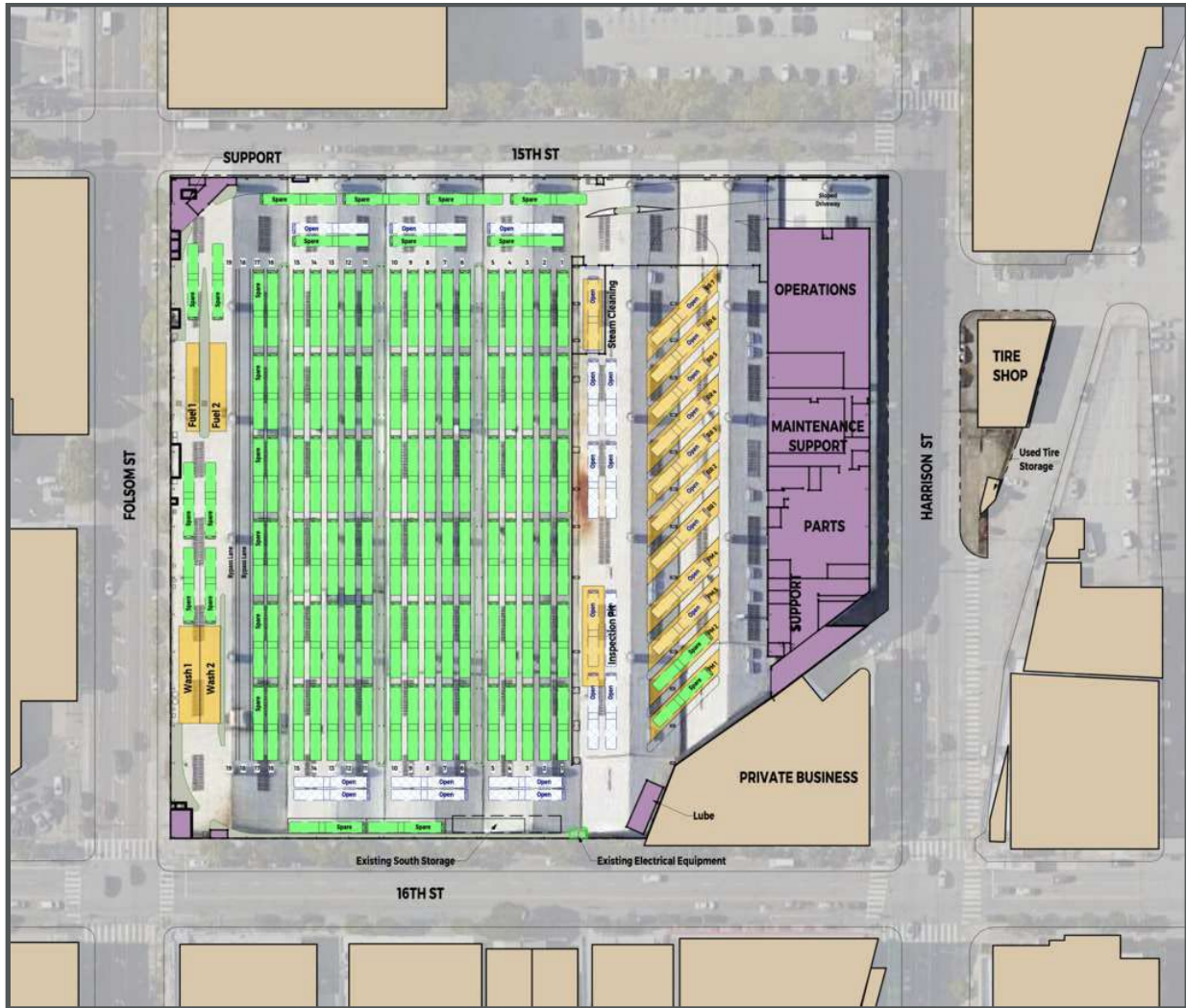
Figure 4-6. Flynn Yard - Existing Conditions (Site Plan)
