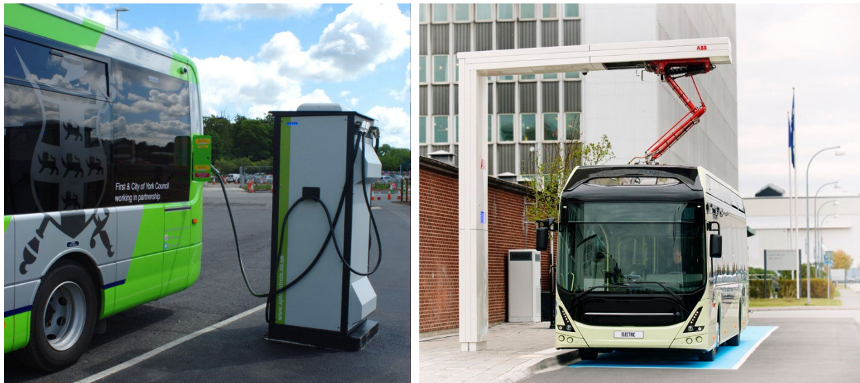
Figure 2-1. Plug-In and Pantograph Charging
