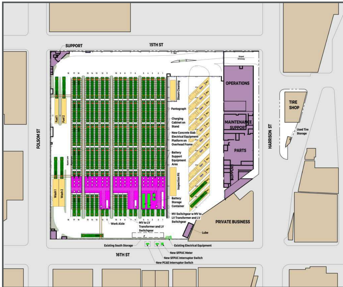
Figure 4-7. Flynn Yard - Full ZEB Build-Out
