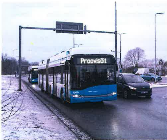
▶ In motion charging trolleybus (Tallinn)
