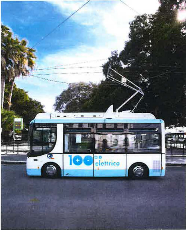
► In motion charging trolleybus (Cagliari)
