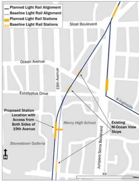
Figure 3-4. Stop Consolidation, Longer and Shorter Subway alternatives
