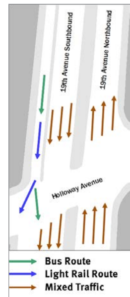
Figure 4-5. Bus/Light-Rail Shared Transitway Operation: Buckingham to Holloway
