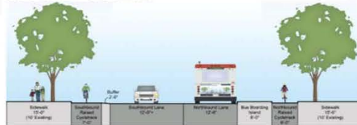
Typical Bus Boarding Island Section
