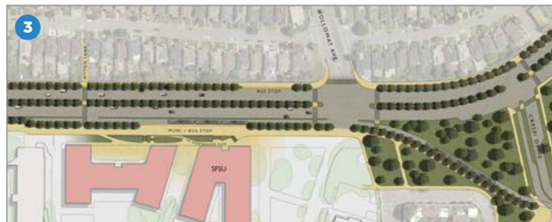
SF State's 19th Avenue frontage, reconfigured with wider sidewalks/bus stops, and a landscaped median.
