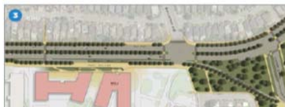
SF State's 19th Avenue frontage, reconfigured with wider sidewalks/bus stops, and a landscaped median.
