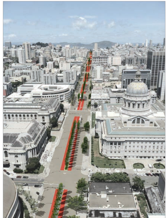
The Van Ness Avenue BRT project features a dedicated center transit lane between Mission and Lombard streets. The transit lane, along with a package of complementary transit and pedestrian improvements, will significantly enhance transit reliability and pedestrian safety.
