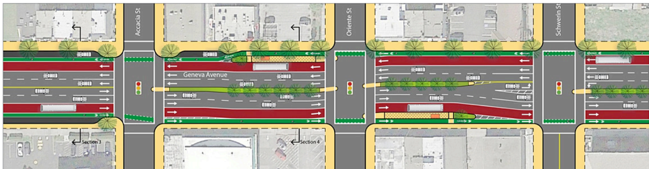
FIGURE 17. PLAN DRAWING OF 4 LANE GENERAL PURPOSE / SIDE RUNNING BRT ALTERNATIVE – ORIENTE STREET STATION
