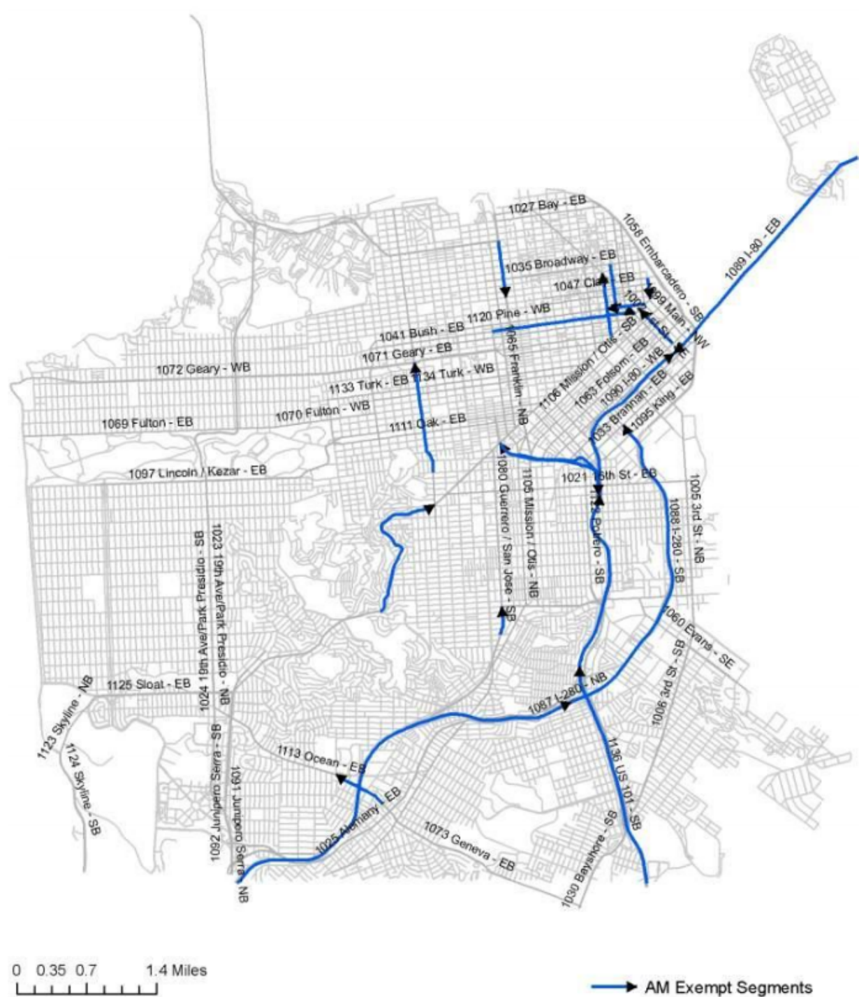
Figure A5-1 Segments Exempt in AM Due to Monitoring at LOS F in Inaugural Cycle
