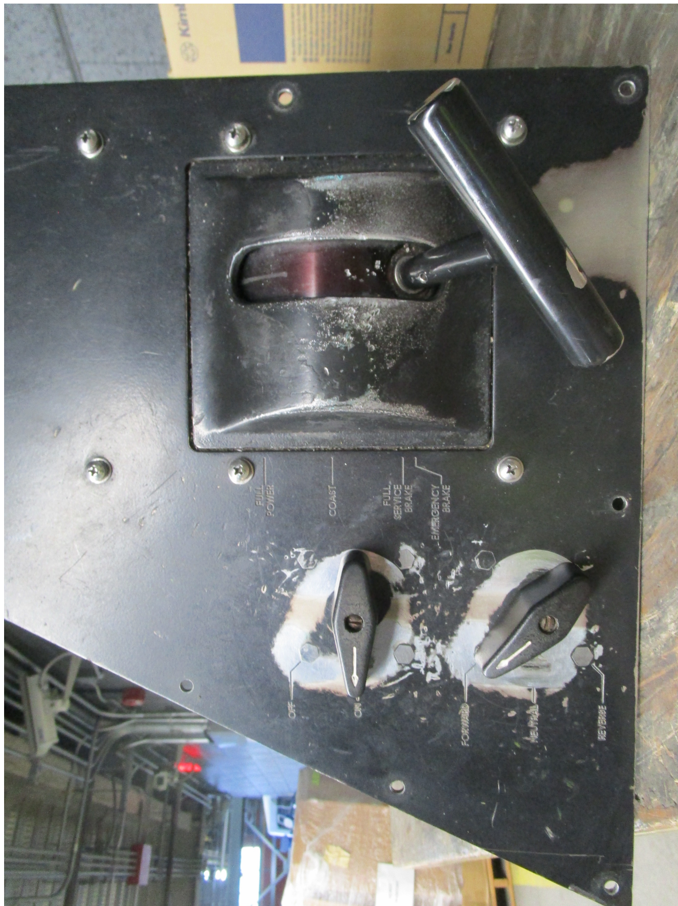
Breda LRV Master Controller - Existing Condition
