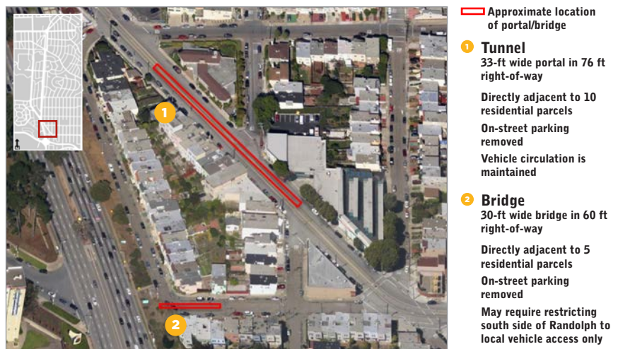
Figure 4-8. Visual, Traffic Circulation Tradeoffs: Tunnel vs. Bridge
