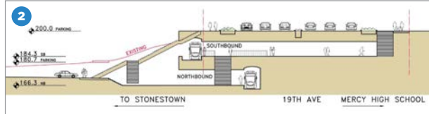
New station between Macy's and Mercy High School with entrances on both sides of the street.
