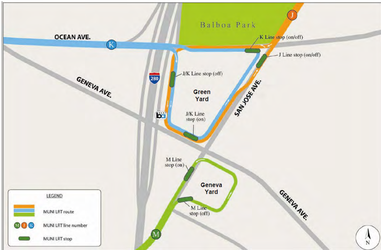
Figure 2: Light Rail Vehicle Circulation at Balboa Park BART Station (Capacity Study, SFMTA, 2011)
