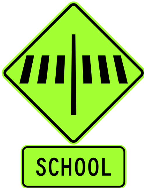
Figure A3-2 High Visibility Signs
