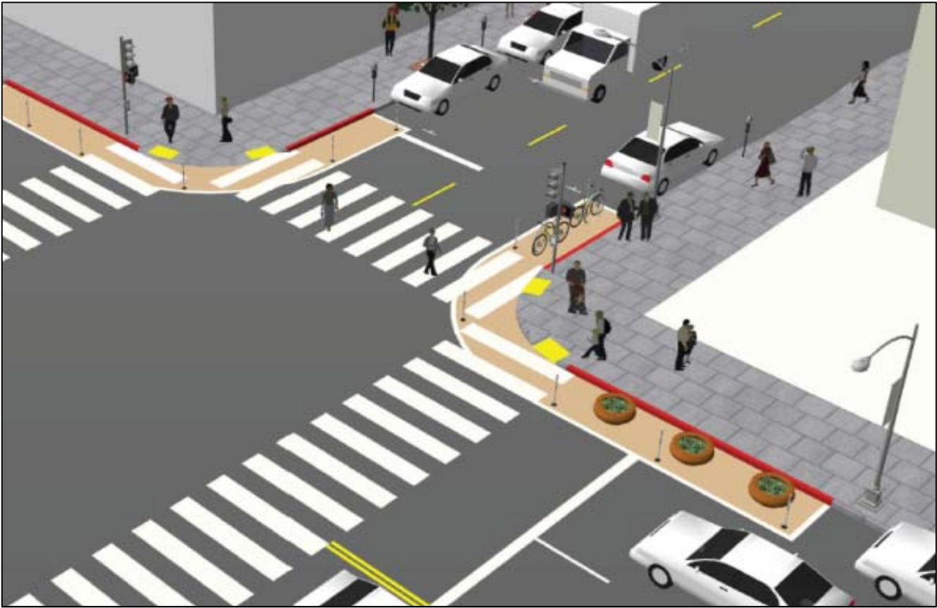
Figure 1. Conceptual drawing of Painted Safety Zones (PSZ) before conversion to permanent concrete bulb-outs.
