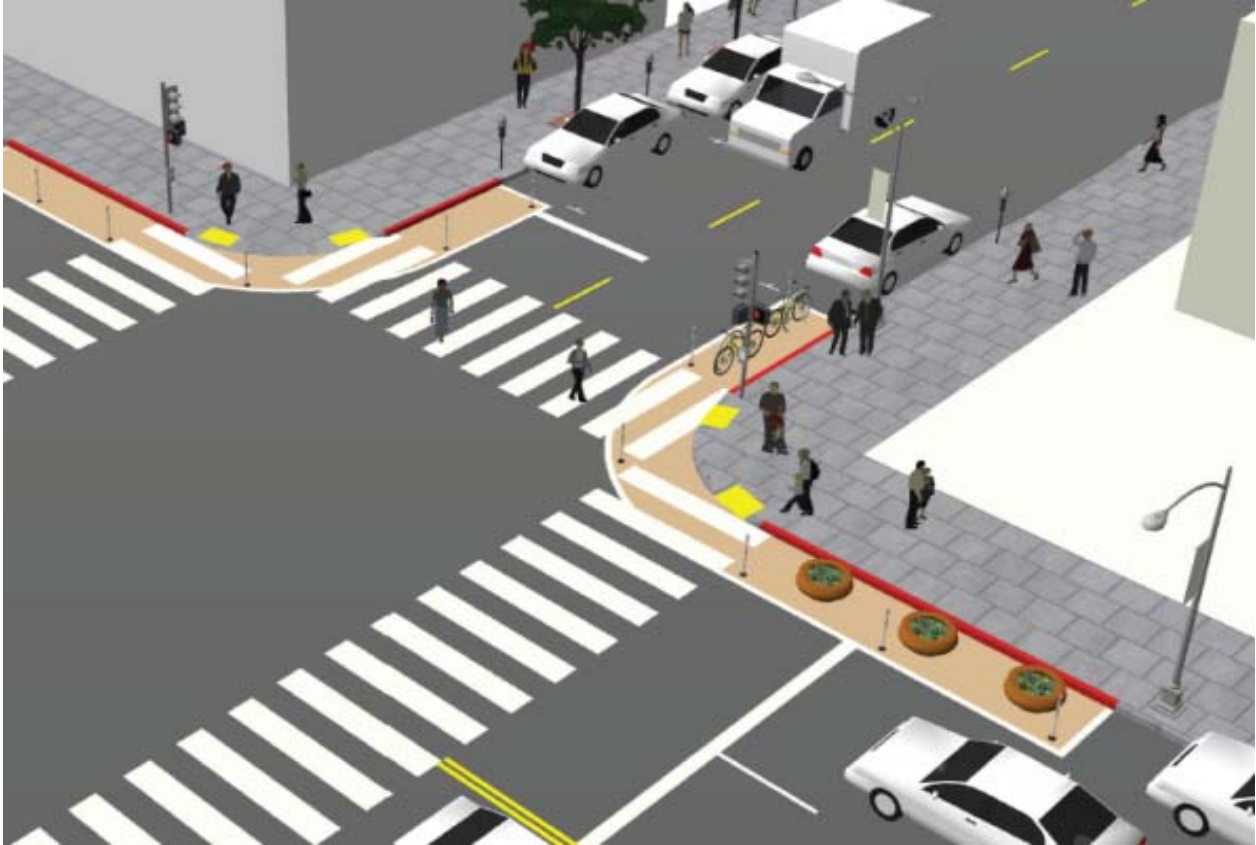
Figure 1. Conceptual drawing of Painted Safety Zones (PSZ) before conversion to permanent concrete bulb-outs.
