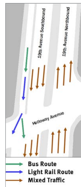
Figure 4-5. Bus/Light-Rail Shared Transitway Operation: Buckingham to Holloway
