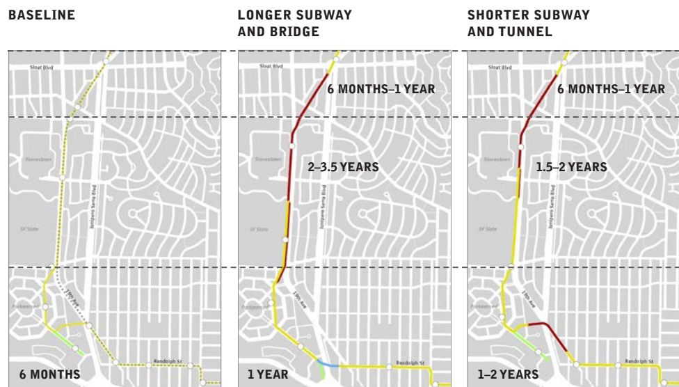
Figure 4-13. Evaluation Results: Approximate Construction Duration
