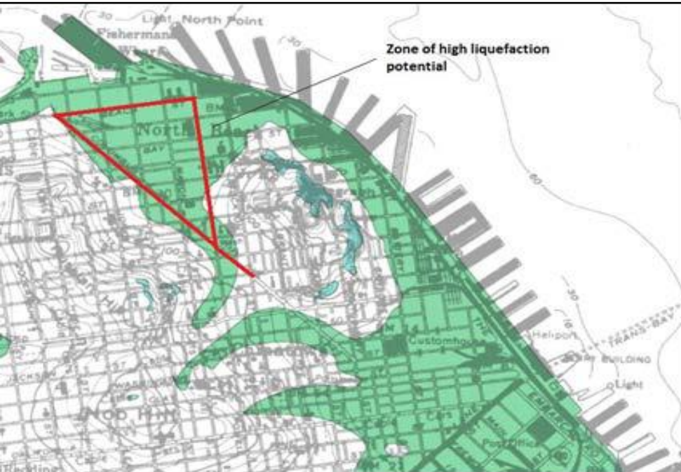
Areas of possible liquefaction
