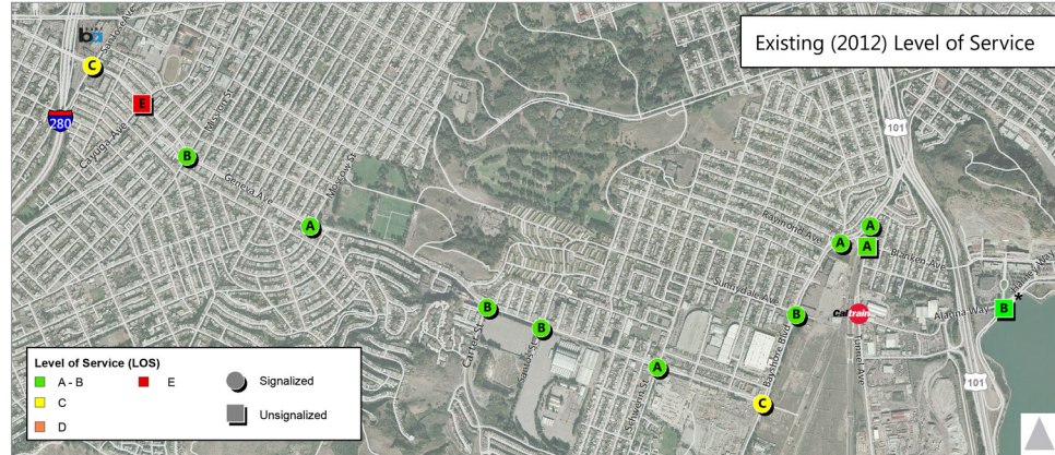
FIGURE 46. EXISTING CONDITIONS - 2012 LEVEL OF SERVICE
