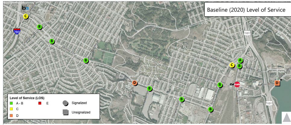
FIGURE 47. BASELINE - 2020 LEVEL OF SERVICE
