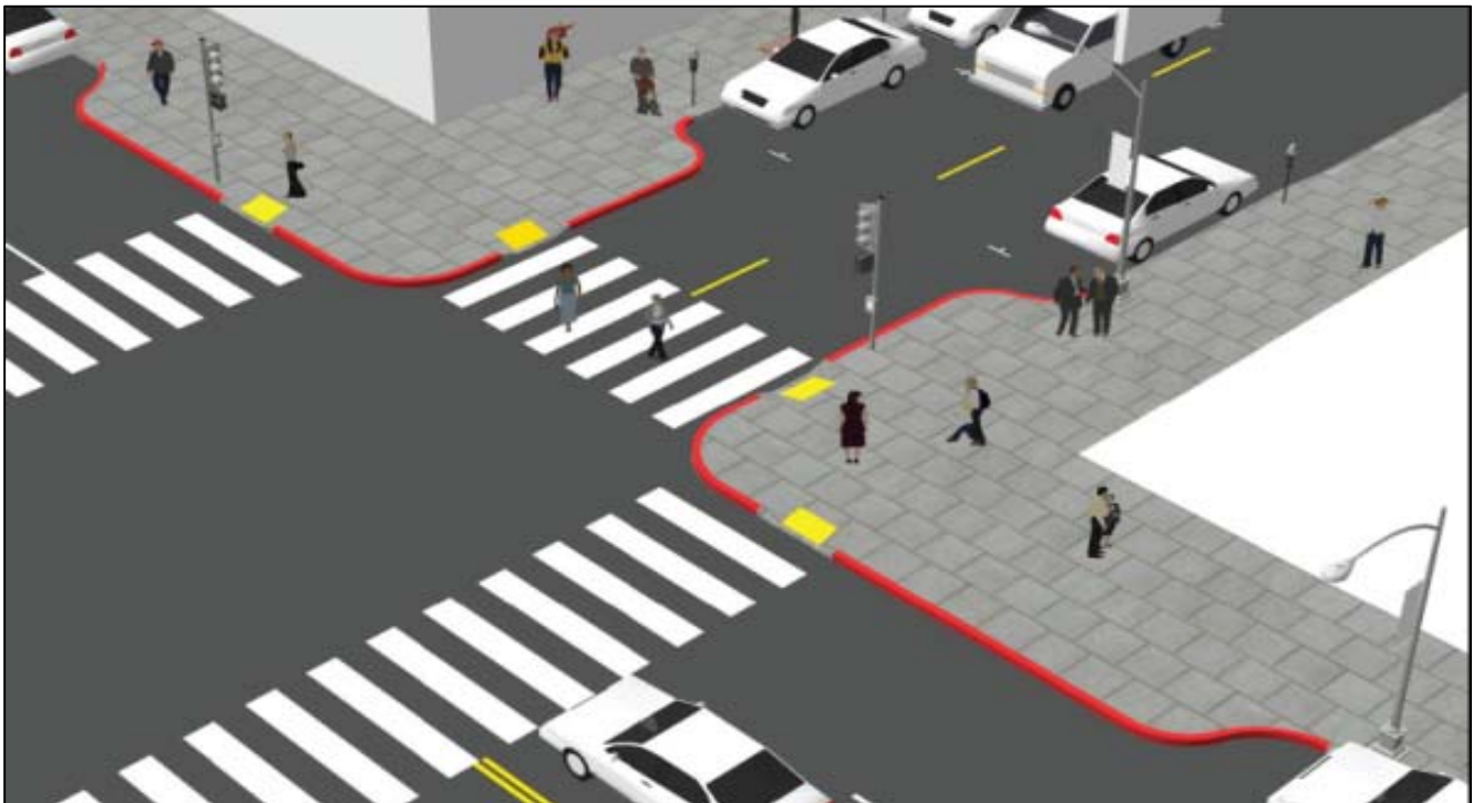
Figure 2. Conceptual drawing of Painted Safety Zones (PSZ) after conversion to permanent concrete bulb-outs.
